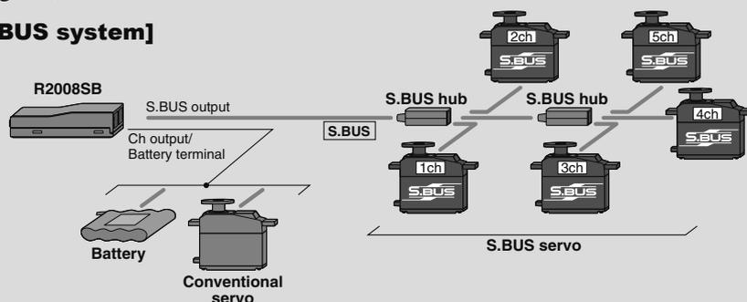
\* Set the channel at the **S.BUS** servos by using an **SBC-1** channel changer or a **CIU-2** USB serial interface.
