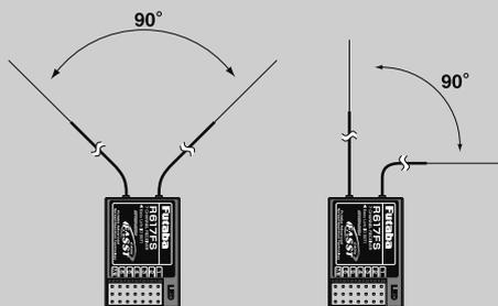
This is not a critical figure, but the most important thing is to keep the antennas away from each other as much as possible.
